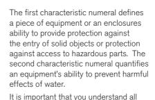
enclosure or equipment is exposed to.
