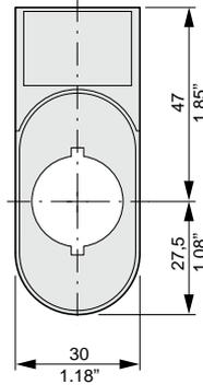
**Mounting drilling with slot**
