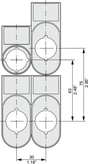
Grid dimension for P SN/DD... with protection cap P SN/T/DD
