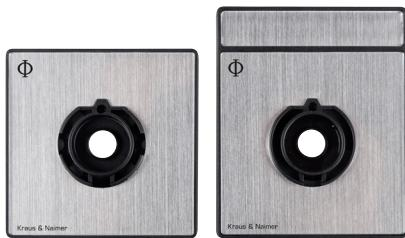
Square and rectangular escutcheon plates are available for each size of switch. The escutcheon plate consists of a frame and a faceplate having the switch positions which is than embossed with hot-foil backing. The escutcheon plate frame is an essential part of the switch and serves as a bearing surface for the handle. If the switch is to be mounted without an escutcheon plate we would recommend for size S1 the handle bearing plate T100-04.
