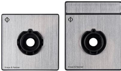
Square and rectangular escutcheon plates are available for each size of switch. The escutcheon plate consists of a frame and a faceplate having the switch positions which is then embossed with hot-foil backing. The escutcheon plate frame is an essential part of the switch and serves as a bearing surface for the handle. If the switch is to be mounted without an escutcheon plate we would recommend for size S1 the handle bearing plate T100-04.
